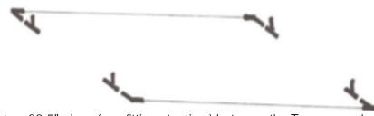
b. Connect two 33.5" pipes (one fitting at a time) between the Tees on each side.
